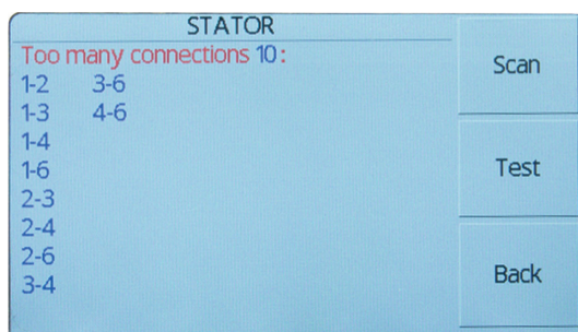
Figure 15 – Detection of phase connection with exceeded number of commutations
